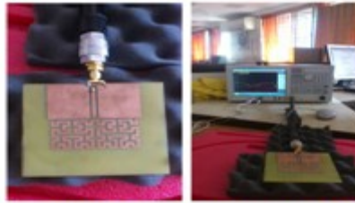
Figure 1.11(b): experimental setup of fabricated Hilbert curve fractal antenna 3 rd iteration
